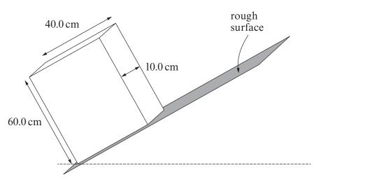
The following diagram shows the block viewed from the side **at the point of toppling**. An arrow is shown passing through the centre of gravity of the block.
